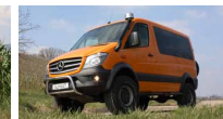
Individual all-wheel drive conversion of a caravan with big wheels, pre-separator, spare wheel holder and bull bar
