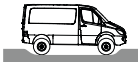
Front angle of driving slope approx. 35° Rear angle of driving slope approx. 31°
