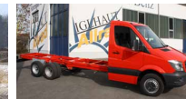
Increase in load capacity up to 7.49 tons by installing a third axle
